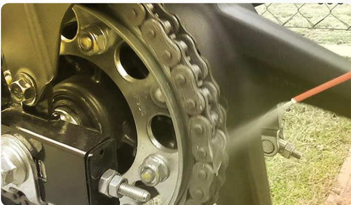
Lubricating the chain
